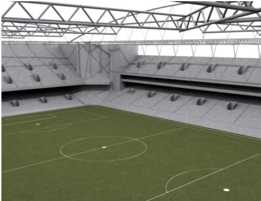
Corner Panelling may be solid or glazed. With TV screen mounted (not shown). (Roof shown transparent)
