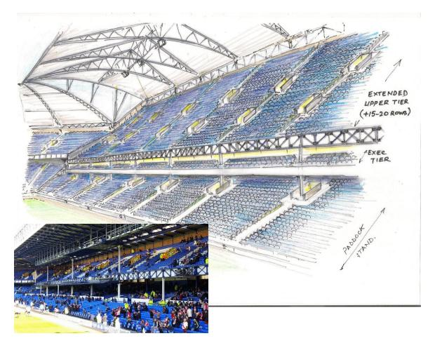
These options would all at least give the impression of preserving the over-lapping format of the traditional double-decker, and with the extension and re-roofing of the upper tier would completely or substantially eradicate obstructions on this side altogether, while at the same time preserving an increasingly rare example of Archibald Leitch's work.
