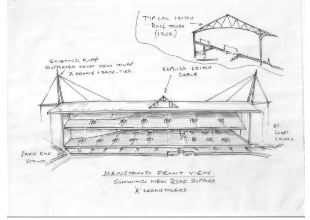
Fig 31. Mainstand with front roof supports removed and back-stays supporting existing segmented roof truss With Replica Leitch Gable on the centre-line.
