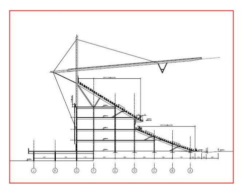
Fig 49. Cross Section South stand (Kirkby), Note: no significant overhang of upper tier.
