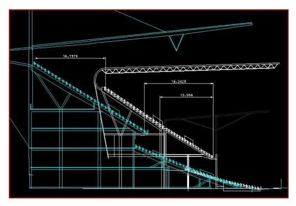
Fig 51. Comparison: Kirkby cross-section superimposed on extended Bullens Rd stand. Note: existing stand position (Grey roof-line).
