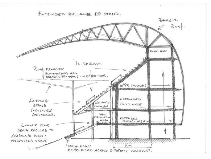
Fig 16. Extended Bullens Rd stand Cross section.
