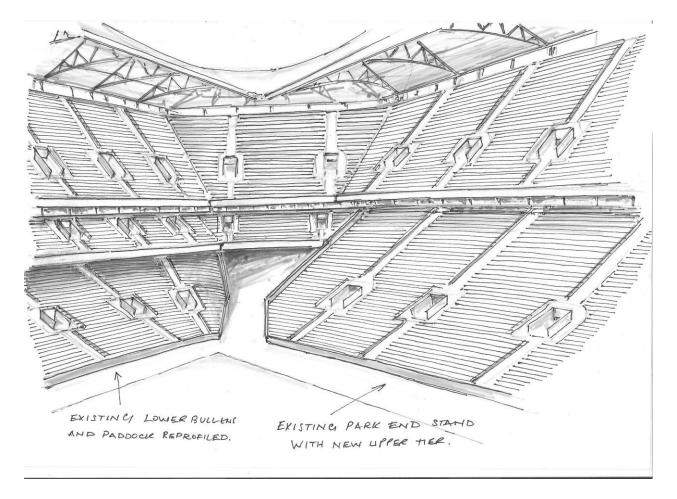
Fig 41. Triple-Tier Bullens with Corner section Joining 2-Tier Park End Stand.
