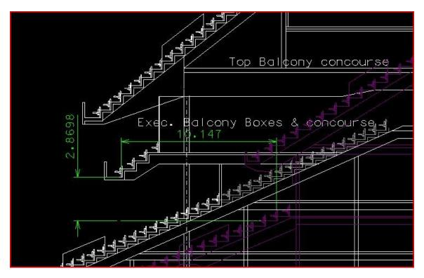
Fig 52. Comparison between Exec box positioning. (Kirkby shown in purple)
