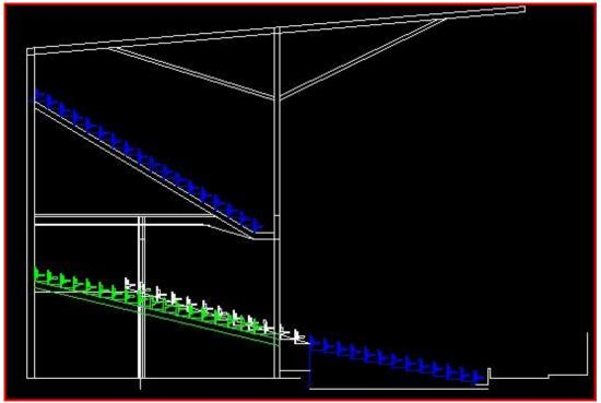
Fig 9. Re-profiled Lower Bullens (green seats are replaced by those shown in white.)
