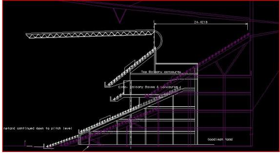
Fig 50. Comparison: Kirkby cross-section superimposed on remodelled mainstand cross-section.
