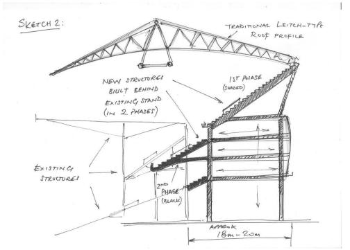
Above: Fig 19. Cross section of new two-tiered Bullens Rd Stand Extension.
