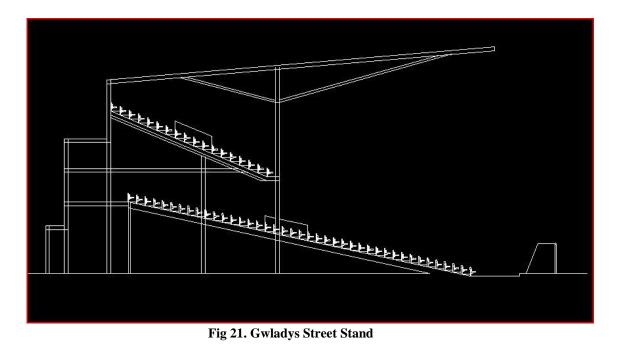
As shown above (fig 21), the Upper Gwladys street stand also has 2 rows of support columns, but this later example of Leitch's work has less supports, and being an end stand also has a narrower viewing range generally. Therefore the removal of just the back 2-5 rows would probably be sufficient to reduce the number of obstructed seats in this stand dramatically, especially those back rows with limited vertical views.
