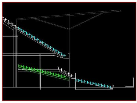
Fig 10. New Lower Bullens Exec tier (seats shown green replaced by those in white)
