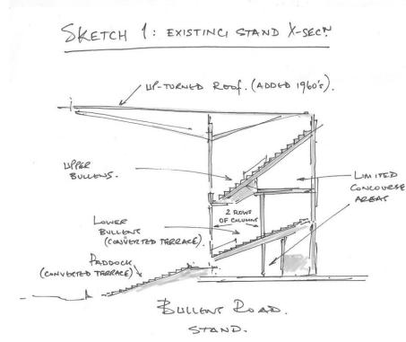
Fig 8. Bullens X-Section
